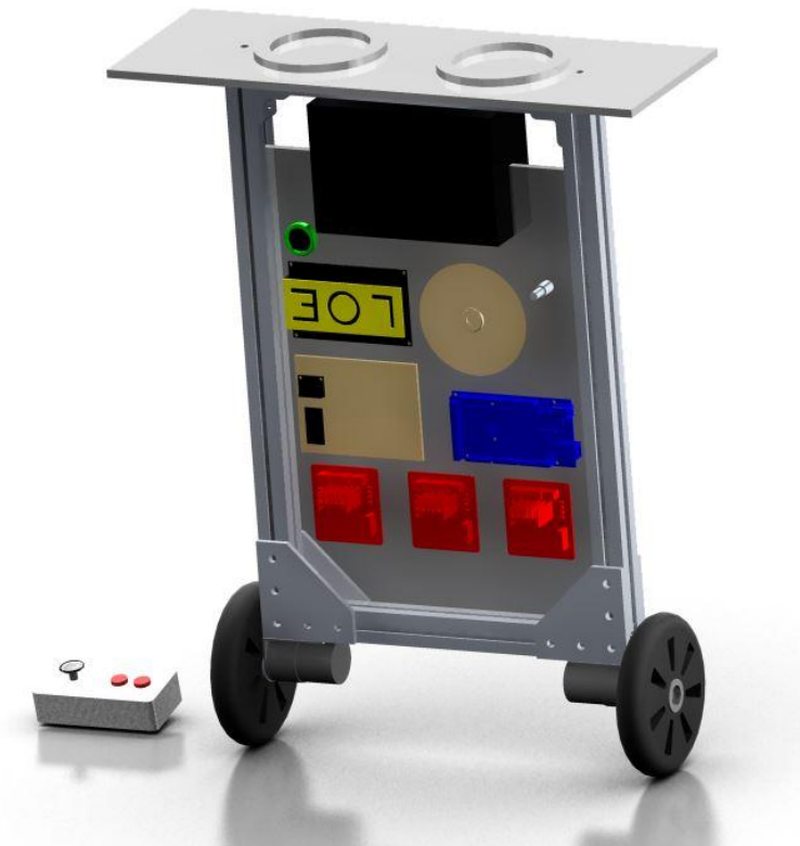
Figure 1 CAD rendered model of the DDV-IP with remote control.
